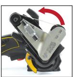
**2** Install Blade Grinding Attachment by aligning the chassis to the keyed "on / off" position then rotate into the "sharpening position".
